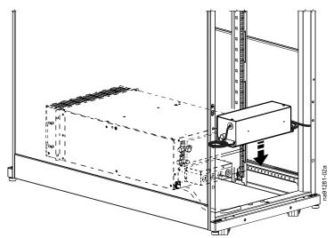
2. Connect the unit condensate drain hose and the pump inlet hose with the copper adapter.
