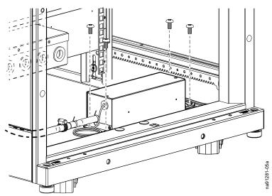
5. Route the 3-m (9.8-ft) long condensate drain tube from the pump out of the unit.
